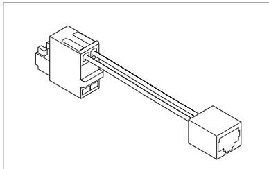
4. 1 Ethernet cable, for example Cat5/Cat6 with external shield, to connect the charging station to the energy meter (not included in the kit).
